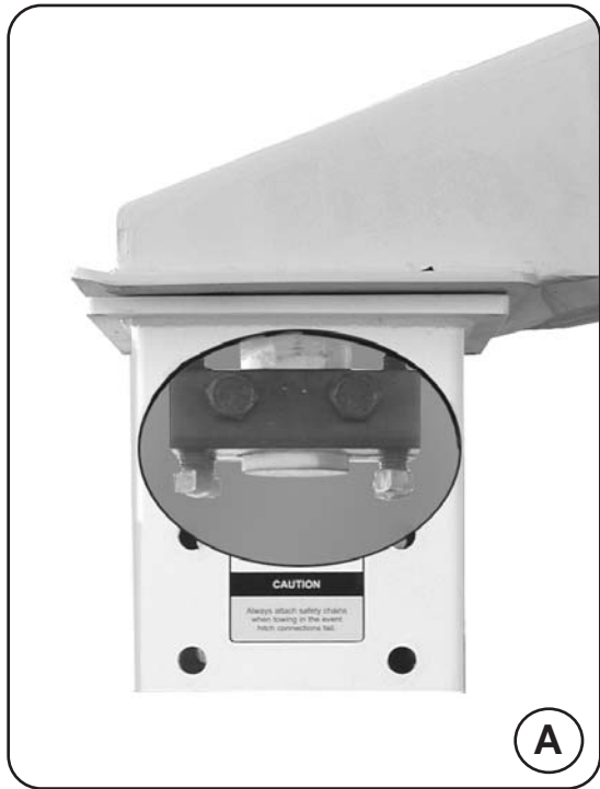
Cutaway view showing King Pin Clamp installed.
